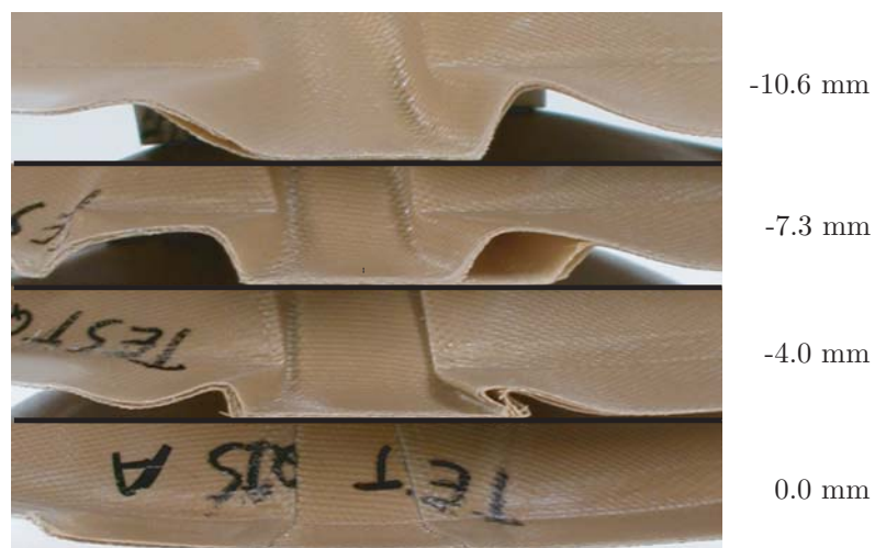
Figure 4.15: Development of wrinkles in a QI laminate at different stages during the rubber pressing process.
